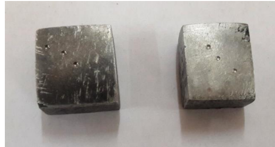
Fig. 12 MMC sample after indentation on hardness testing machine
