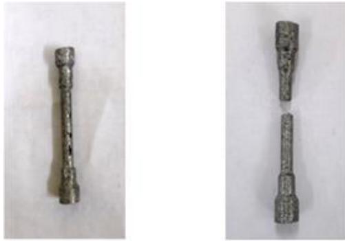
Fig 5 Sample of MMC (a) Before Testing (b) After Testing
